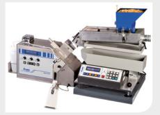
The unique MZ 2000 counting & filling system enables economical and gentle handling of your seeds. The roller conveyor allows the device to operate without vibrations, preventing a separation by size and weight. Additionally, impurities such as glumes of grains and small breakage fragments are removed mechanically.
